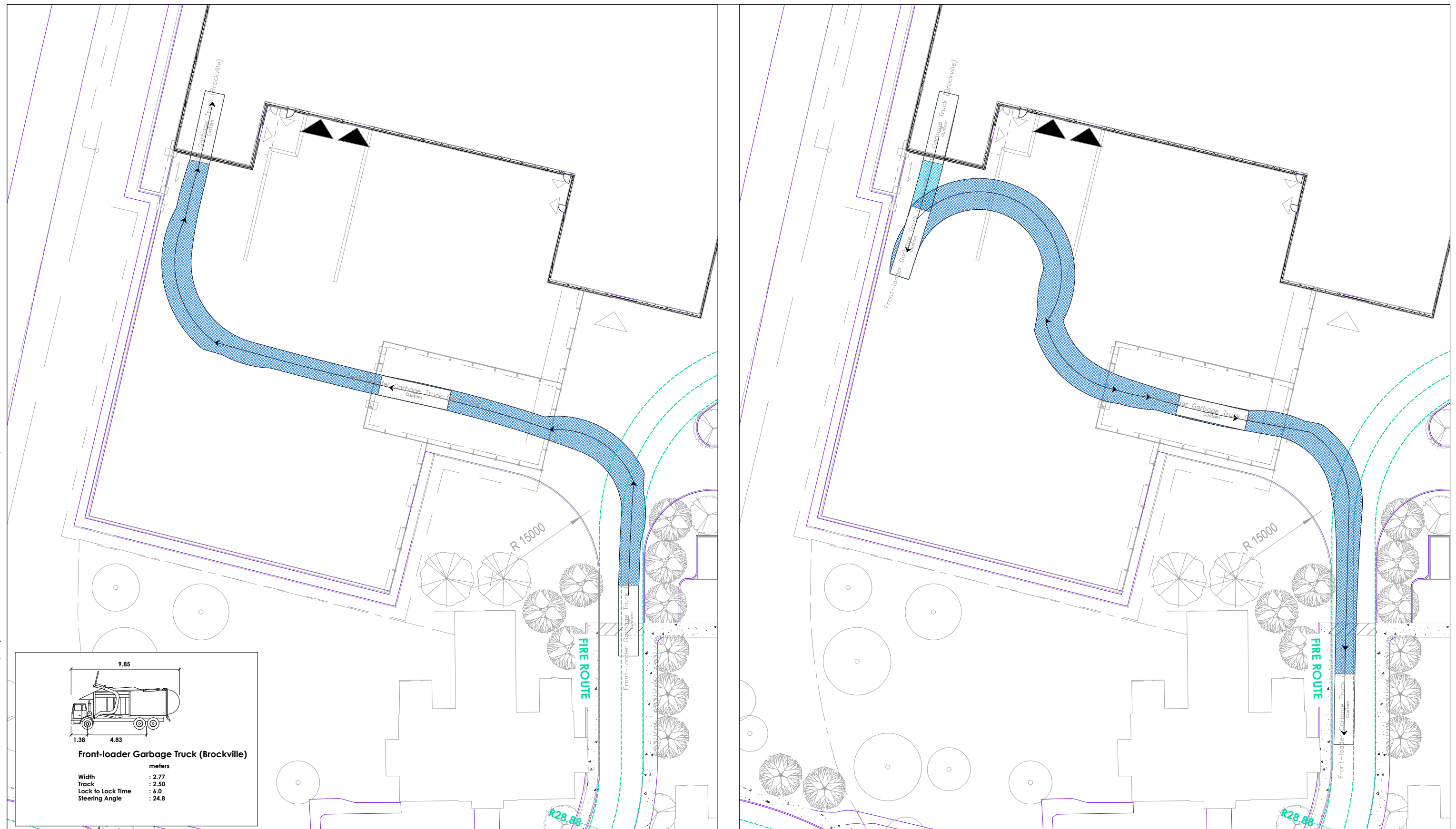
Figure 7-18 Garbage Truck Loading Bay Access Manoeuvre Review Brockville Correctional Complex
