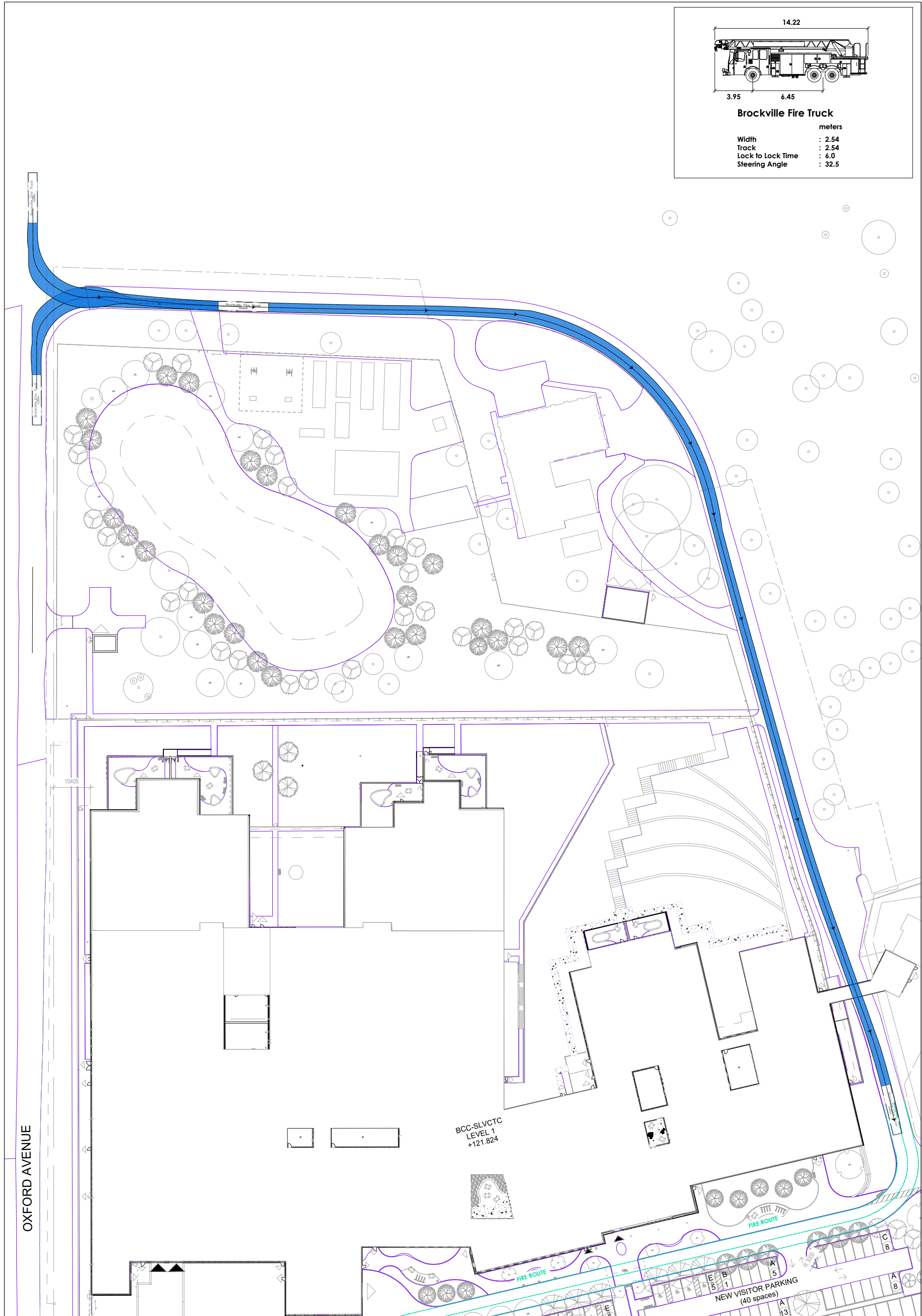
Figure 7-12 Fire truck Turning Manoeuvres at Site Access #2- Inbound Brockville Correctional Complex
