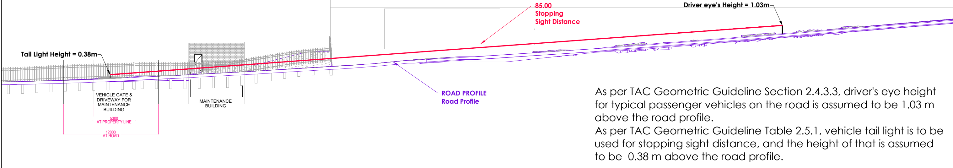
Figure 7-8 Stopping Sight Distance Review (Road Profile) - Maintenance Building Driveway Intersection at Oxford Ave Brockville Correctional Complex
