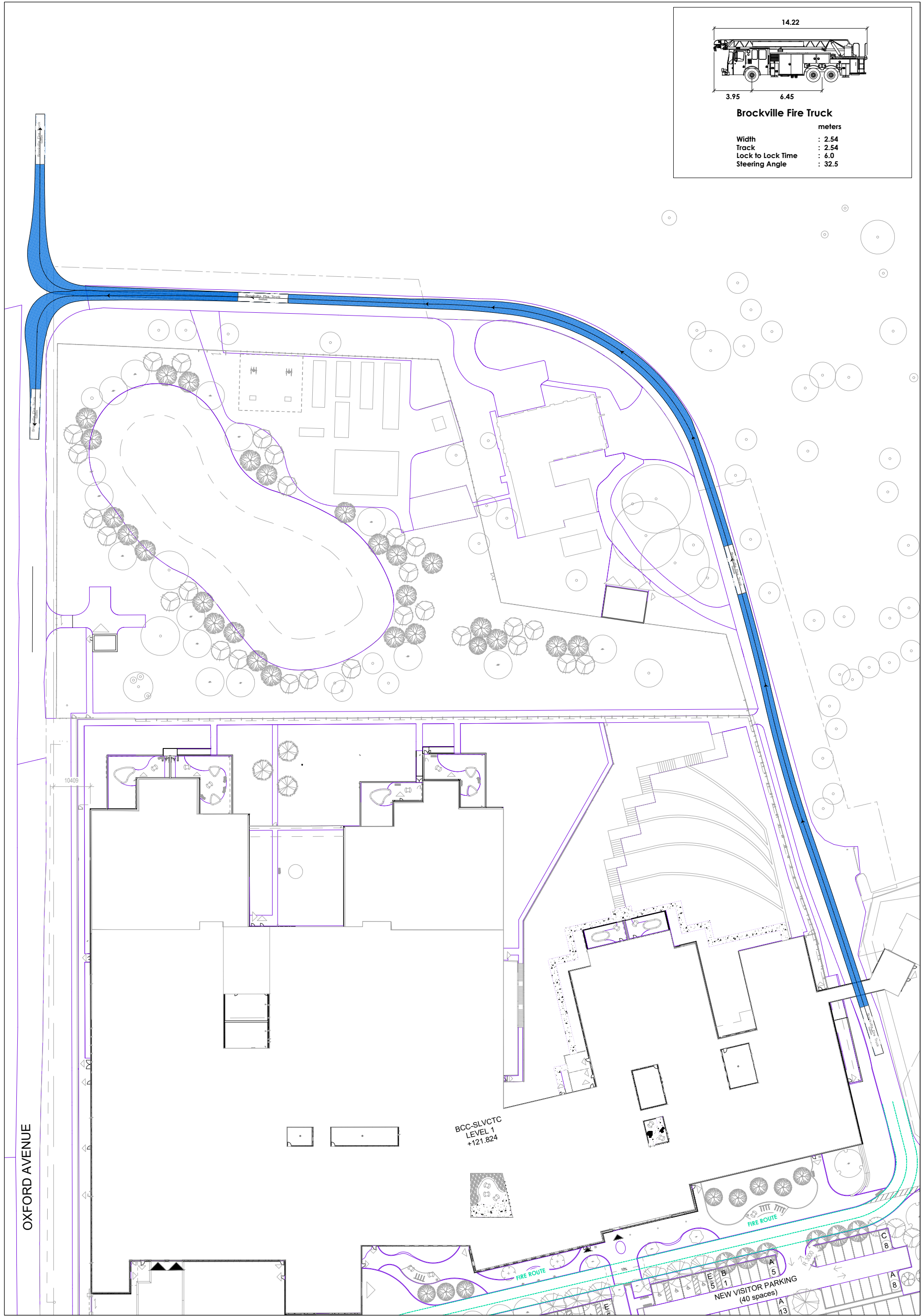
Figure 7-13 Fire truck Turning Manoeuvres at Site Access #2- Outbound Brockville Correctional Complex
