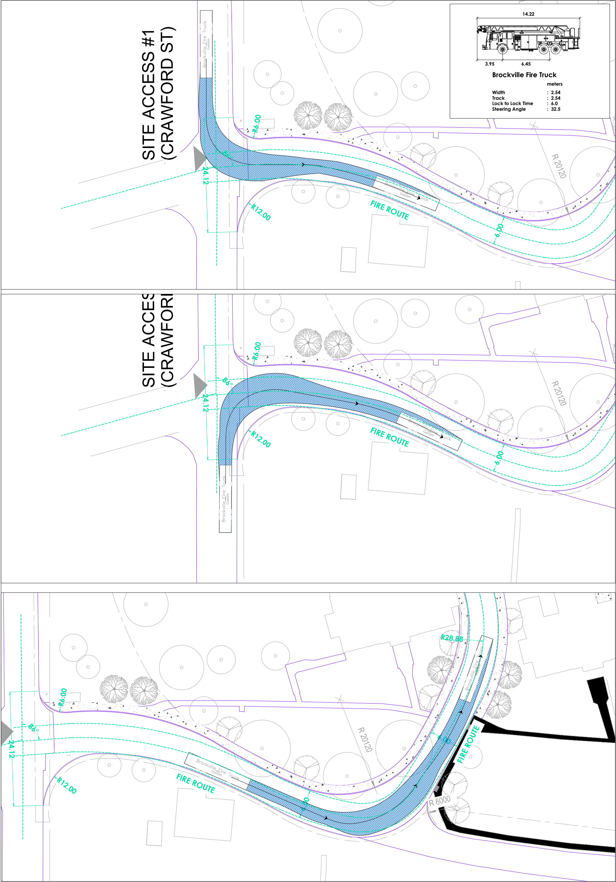
Figure 7-10 Fire truck Turning Manoeuvres at Site Access #1 - Inbound Brockville Correctional Complex
