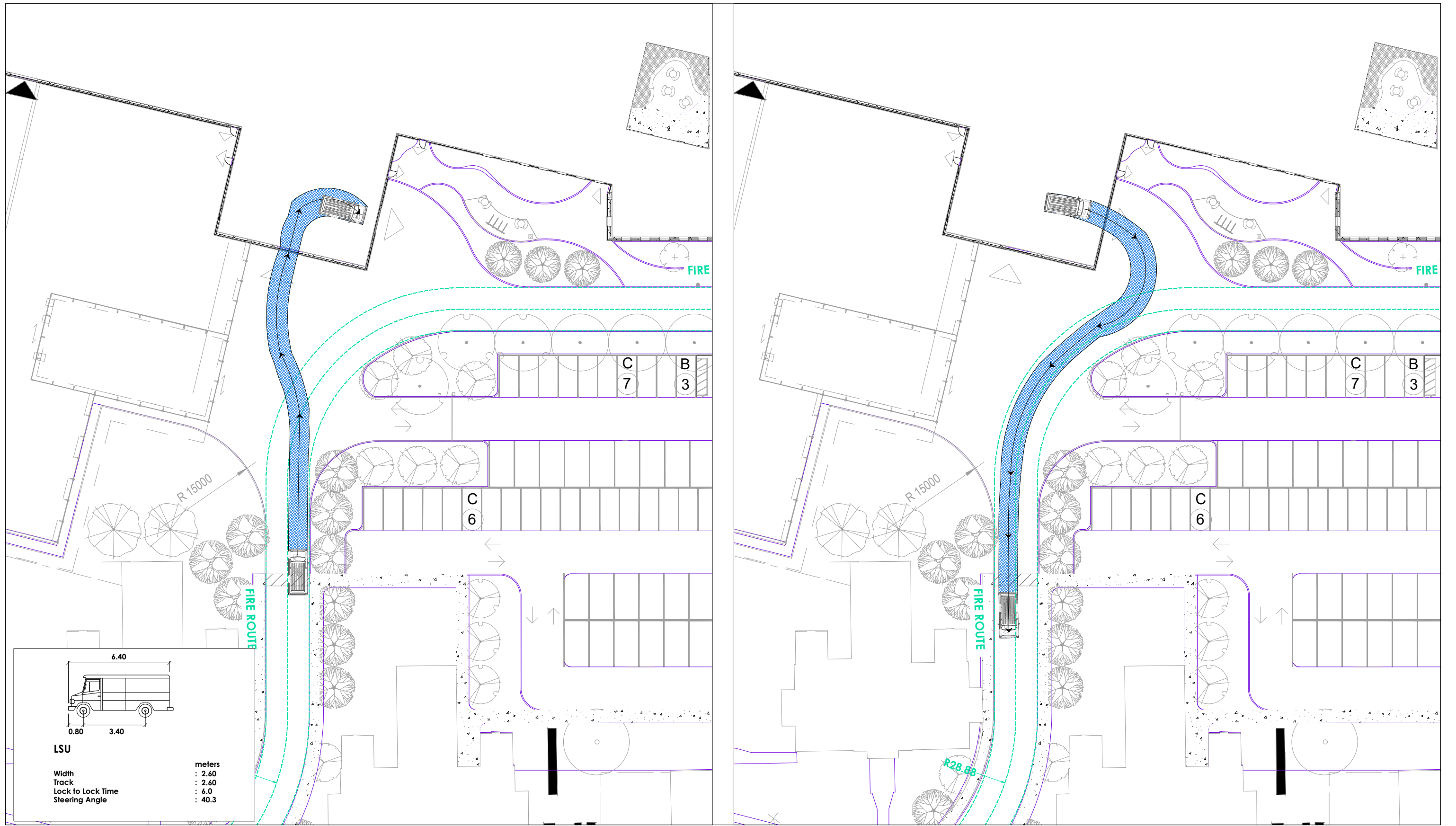
Figure 7-23 Delivery Truck Access Manoeuvre Review Brockville Correctional Complex
