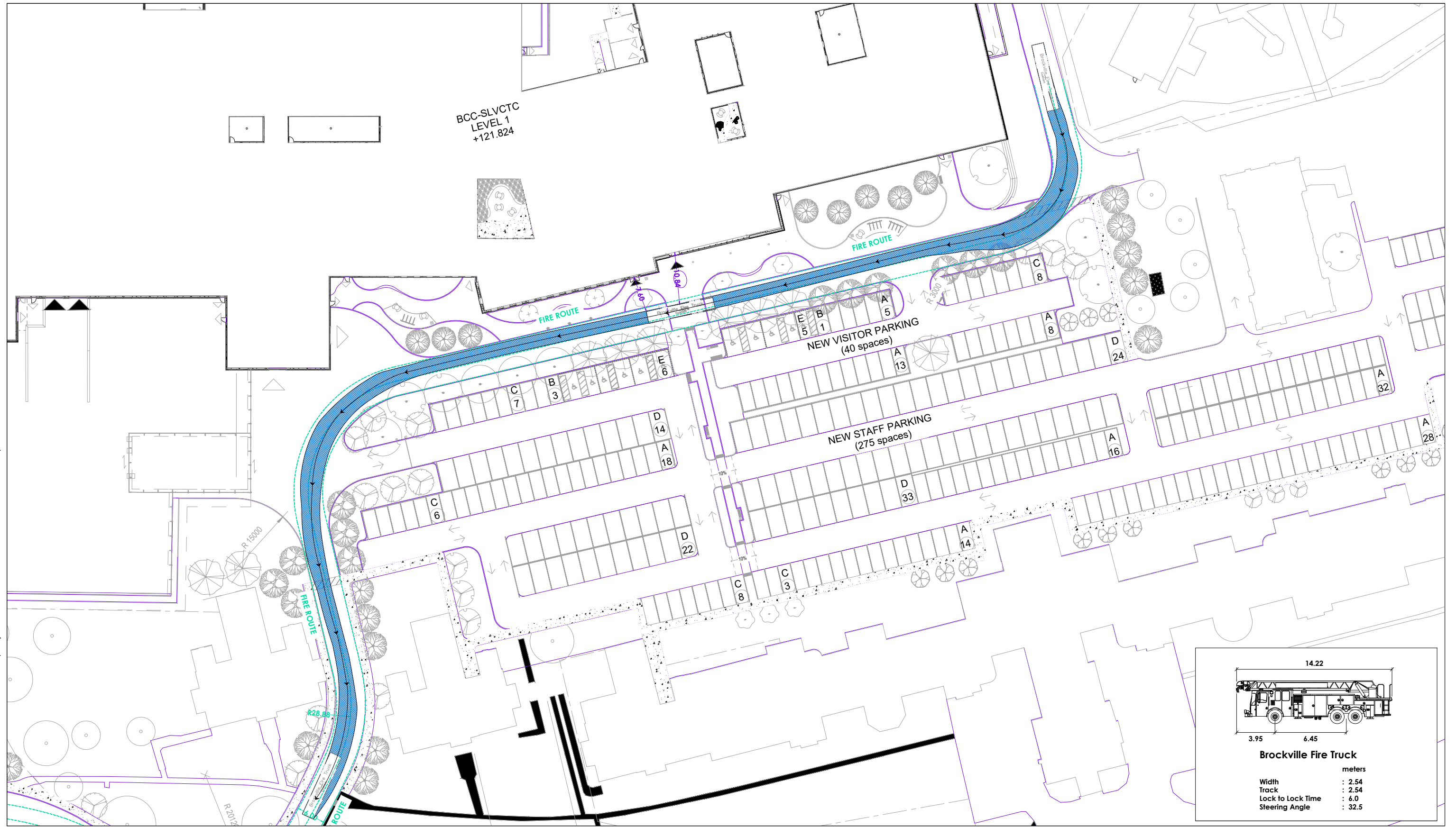
Figure 7-15 Fire Truck Site Circulation Manoeuvre Review - from Site Access #2 Brockville Correctional Complex
