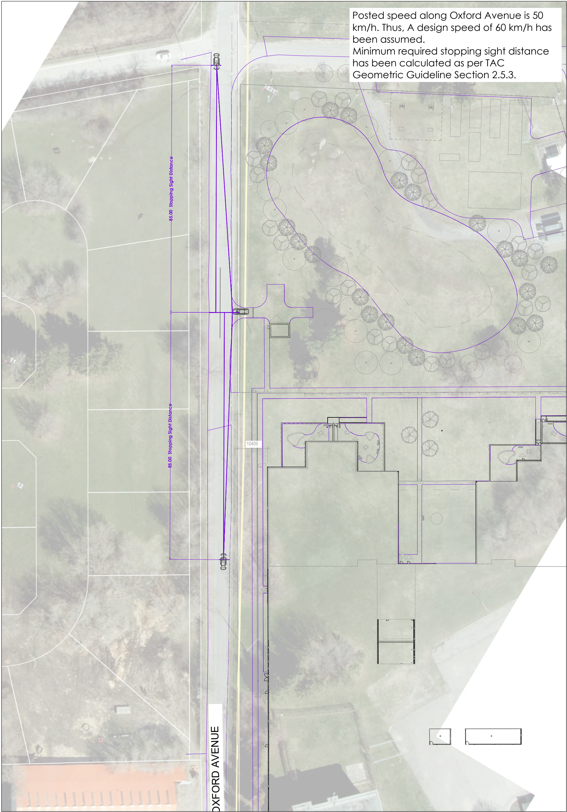
Figure 7-6 Stopping Sight Distance Review - Maintenance Building Driveway Intersection at Oxford Ave Brockville Correctional Complex
