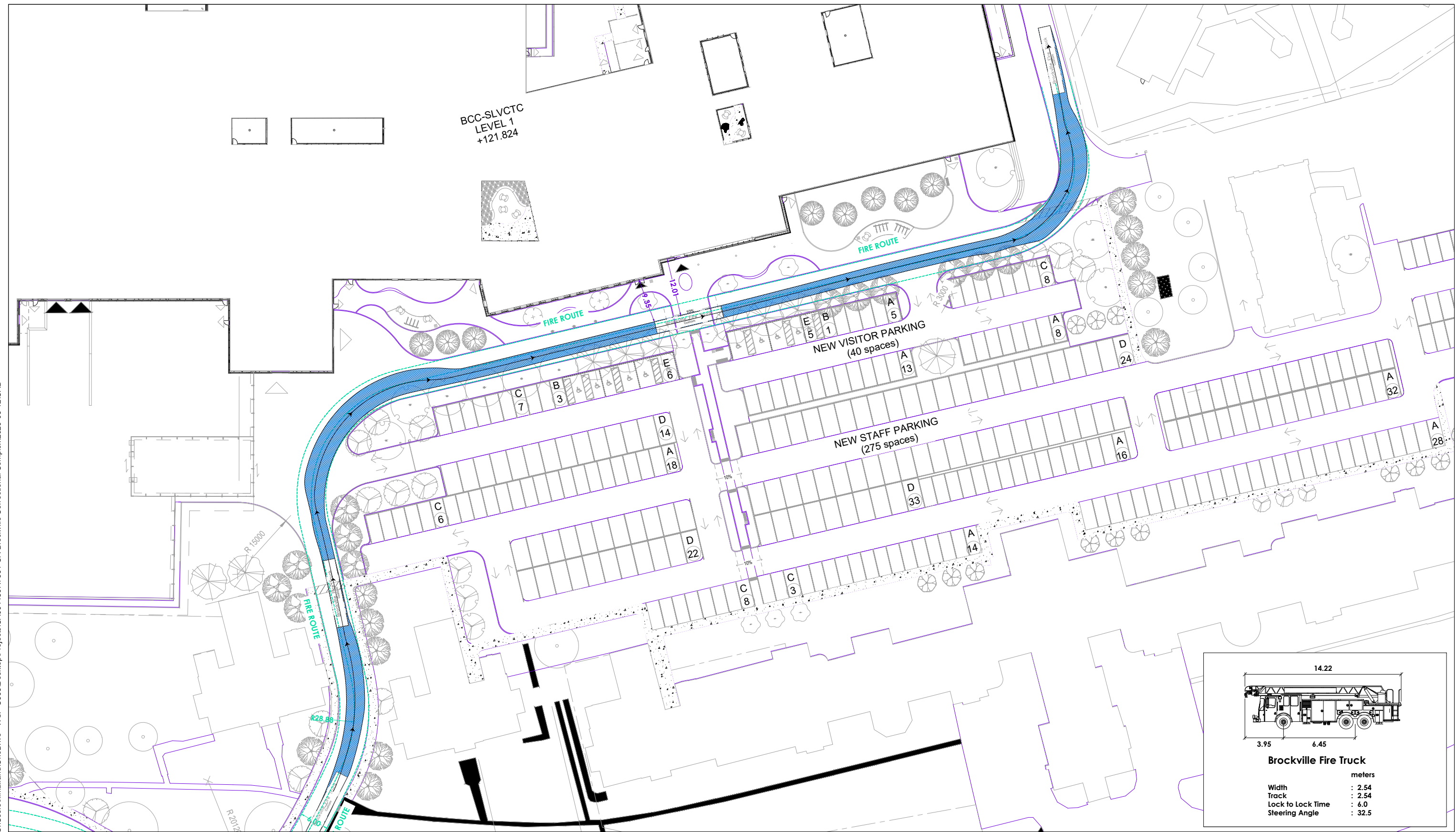
Figure 7-14 Fire Truck Site Circulation Manoeuvre Review - from Site Access #1 Brockville Correctional Complex
